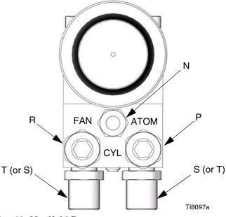
Fig. 10: Manifold Ports
